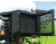
progressively warmer air is drawn through, cool air is available to each core in a single pass, resulting n substantially improved cooling performance.
